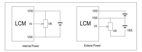
V<sub>DD-</sub>V<sub>0</sub>: LCD Driving voltage VR: 10k~20k
